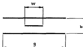
Fig. 1. Strip transmission line.
